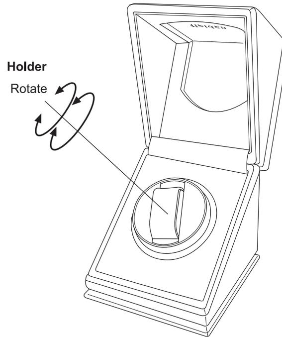
The C-watch holder can rotate a maximum weight of 1/3 pound - operated under a 6V transformer.
